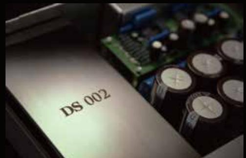
Each lead of every electrical component in the DS 002 is mechanically fixed before soldering and special wiring is added to every signal line on the printed circuit board. These steps are taken to provide the cleanest, shortest signal path in the DS 002 circuit. Every step may be a small improvement, but when added together brings us closer to perfection.
